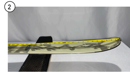
STEP 2: Pull tape measure directly from the tail to mounting location. Do not follow the curvature of the ski, a straight line from tail to midsole is correct.
