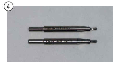
STEP 4: Select the right drill bit. Skis with Titanal in the binding region should be drilled with a 4.1mm x 9.5mm drill bit. Skis without Titanal in the binding region should be drilled with a 3.6mm x 9.5mm drill bit.
