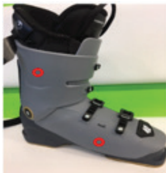
Red circles indicate area temperature was recorded on the shell and cuff.
