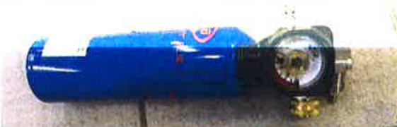
refill-able pressure gas cartridge with valve (including pressure gauge) and cylinder
