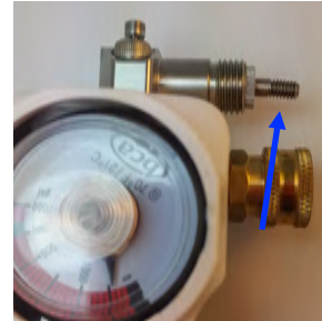
Figure 9: ✖ Bent trigger pin and bad gauge
