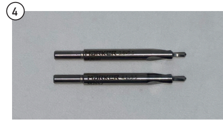
STEP 4: Select the right drill bit. Skis with Titanal in the binding region should be drilled with a 4.1mm x 9.5mm drill bit. Skis without Titanal in the binding region should be drilled with a 3.6mm x 9.5mm drill bit.
